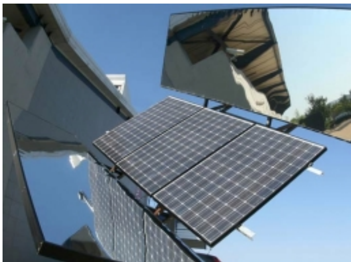
Two reflectors static concentrator 1.8 C
